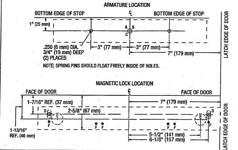
NOTE: FOR MACHINE SCREW MOUNTING, REINFORCEMENT AND STRUCTURING ARE REQUIRED TO WITHSTAND A 1200 LB (544 KG) LOAD. CLEARANCE HOLES FOR FILLER PLATE TO BE SPOTTED AT JOB SITE. CAUTION: "DO NOT ATTACH MOUNTING PLATE TO FILLER PLATE ONLY!"
