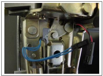
• STRAIN RELIEF WIRES TO EXISTING HOLE IN CENTER CASE. USE THE WIRE CLAMP AND SELF-TAPPING SCREW PROVIDED WITH TRIM.
