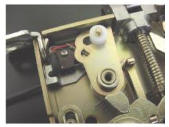
NOTE: MAKE SURE THAT THE FIRE DOOR FUSE GOES THROUGH THE HOLE IN THE AE BRACKET. THIS PROPERLY TRAPS THE BRACKET IN POSITION.
