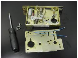
STEP 2: REMOVE TOP LEVER/KNOB HUB AND LOCKING BAR ASSEMBLY.
