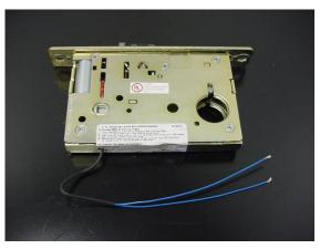
**STEP 1**: REMOVE 5 EACH COVER SCREWS AND REMOVE COVER.
