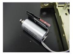
AFTER LOCKING BAR ASSEMBLY HAS BEEN INSTALLED ONTO SOLENOID PLACE THE SOLENOID BACK INTO THE LOCK CASE. THE LOCK CASE TOGGLE NEEDS TO BE POSITIONED IN THE CORRECT SLOT IN LOCKING BAR. MAKE SURE THAT THE WIRES ARE LOCATED ON THE BOTTOM OF THE LOCK CASE SO THAT THEY DO NOT INTERFERE WITH THE SOLENOID AND LINKAGE. FOLD THE EXCESSS WIRE ONTO THE TOP OF THE RECTIFIER IN THE CORNER OF THE LOCK CASE.
